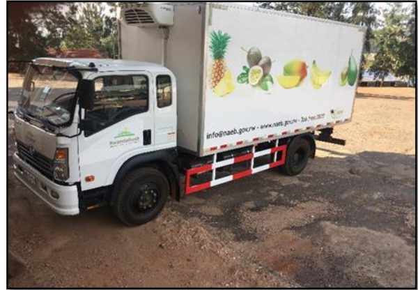
Ishusho ya 725: Imodoka ifite uburyo bwo gukonjesha itwara umusaruro ku rugendo rugufi kuva ku nzu ipakirirwamo umusaruro werekeza ku Kibuga cy’indege © Shivachi
